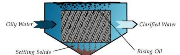
bottom to some degree. Due to oil typically being lighter than water, they (oil) will rise up the coalescing plate. As the oil droplets rise up the plate they will coalesce or come together with other droplets, creating progressively larger droplets. Once the droplet size is sufficient or the droplet reaches the top of the media plate the droplet pulls away from the plate and rises to the water surface. To some degree, the solids replicate this process in reverse (settling).
