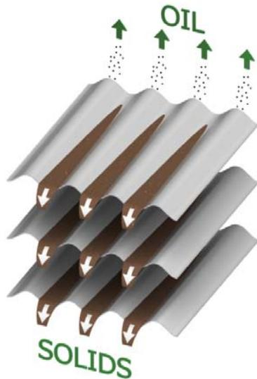
This plate system makes the TPI the best choice when an application has high solids and oil/fuels mixed together in the same wastestream.
